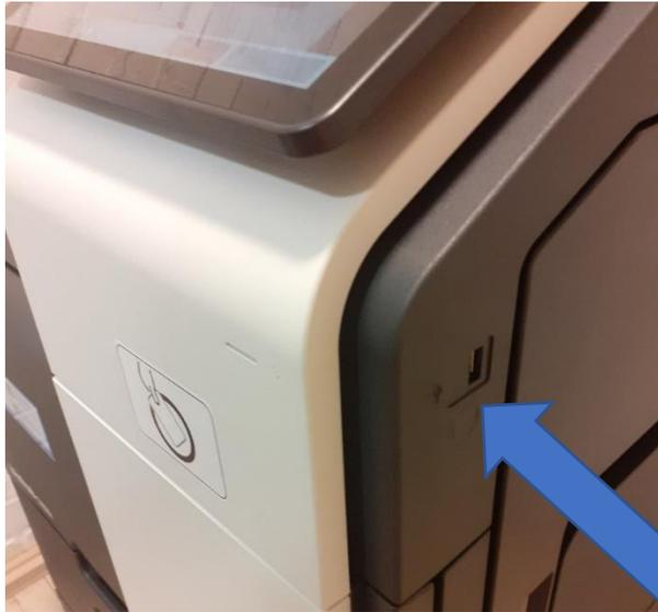
There is a USB port on the right side of the machine if you wish to print from, or scan to, a USB device
